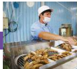
The Ukon is lifted on a conveyor belt where soil and any other impurities are sprayed off.
