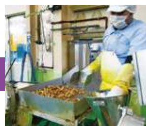
The Ukon is washed through a hot shower and slice it to the thickness of one millimeter and spread to a tray.
