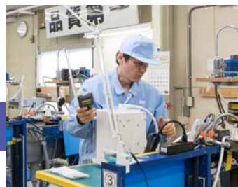
pH testing is also done during water flow testing on the completion line.
