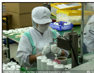
Leak Test: At this stage, the filter is individually inspected for any leaks.
