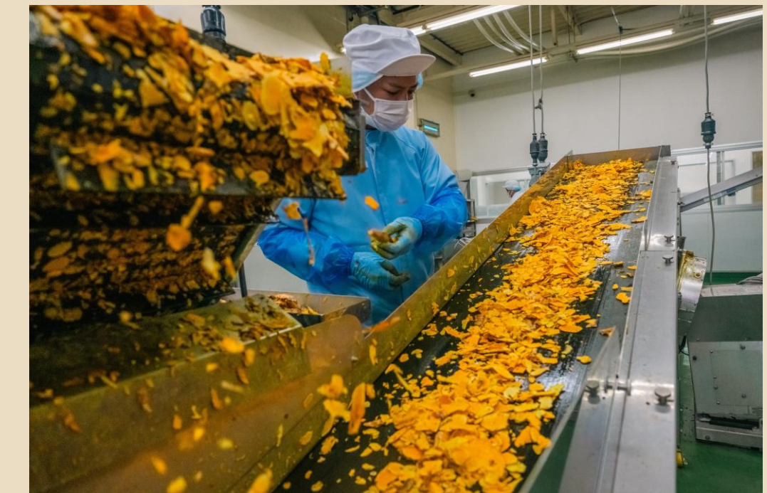
6. Sliced turmeric passes through a conveyor and enters dryer.
