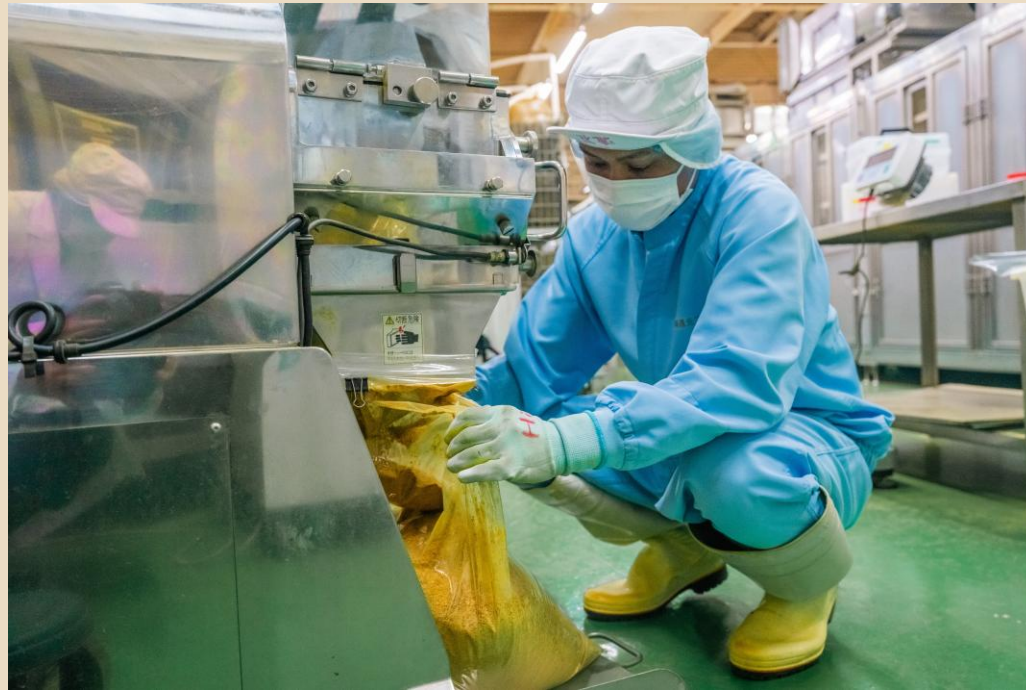
7. Dried turmeric chips are transported by an air conveyor and powdered.
