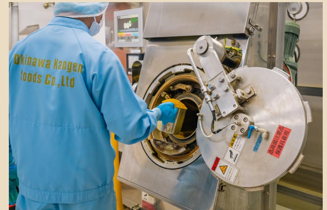
9. Autumn turmeric powder used to make Ukon tea is sterilized in a sterilizer.
