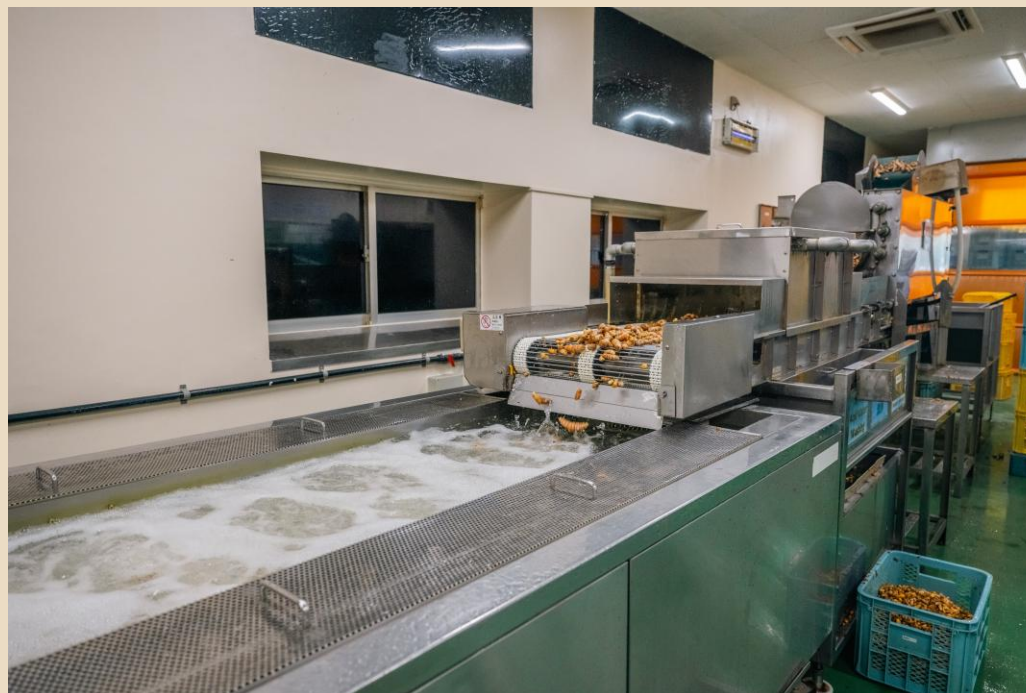
4. Rinse away dirt with high-pressure water.
