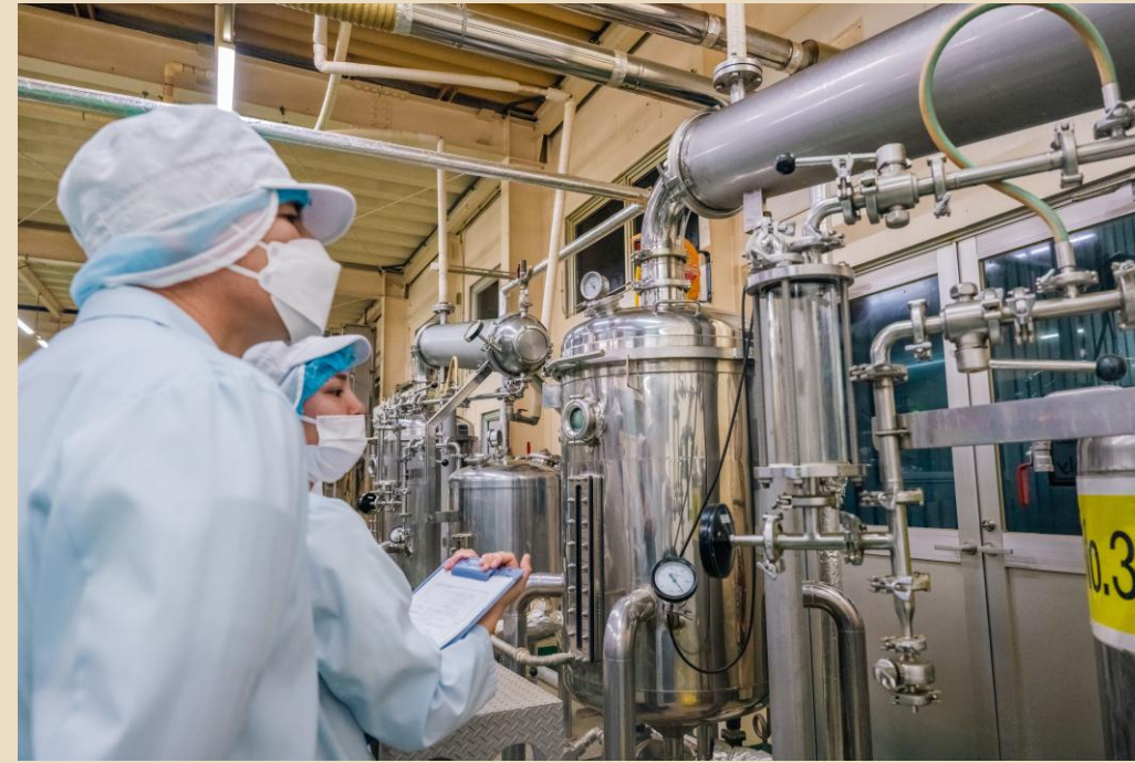
8. Coarsely powdered turmeric is put through a distiller to extract spring and autumn turmeric oil, used in the supplements and soap.
