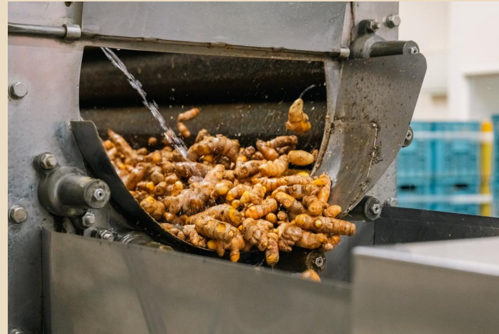
2. Super 501s are used for cleaning and sterilization. Peeling turmeric will help reduce soil bacteria.
