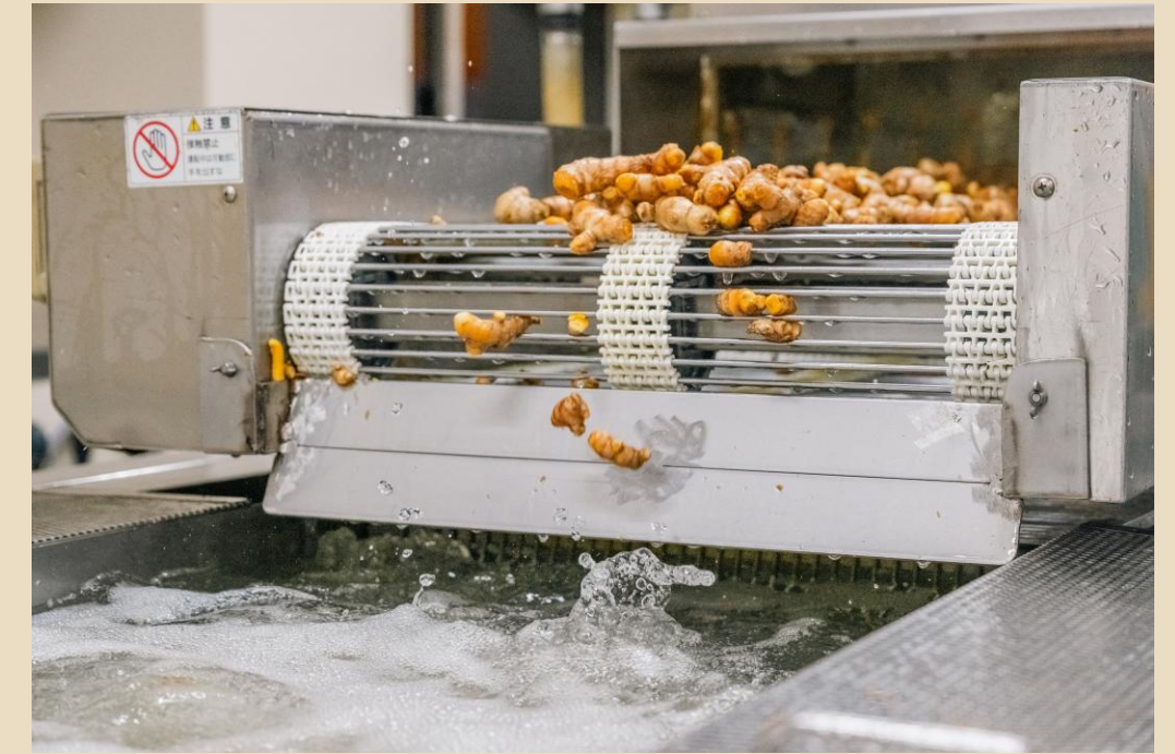
3. Washing with strong acidic water through a low-pressure shower tunnel.
